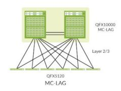
Figure 1: QFX10000 modular switches can be deployed in IP fabric or MC-LAG configurations.
