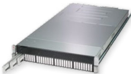
SSG-2029P-DN2RR32L 2U SBB with 32 Intel® "Ruler" SSDs
